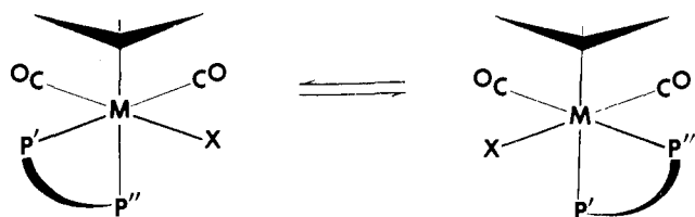
Figure 5. The trigonal twist rearrangement proposed for (\eta^3\text{-C}_3\text{H}_5)\text{M}(\text{CO})_2(\text{P-P})\text{X} complexes.
